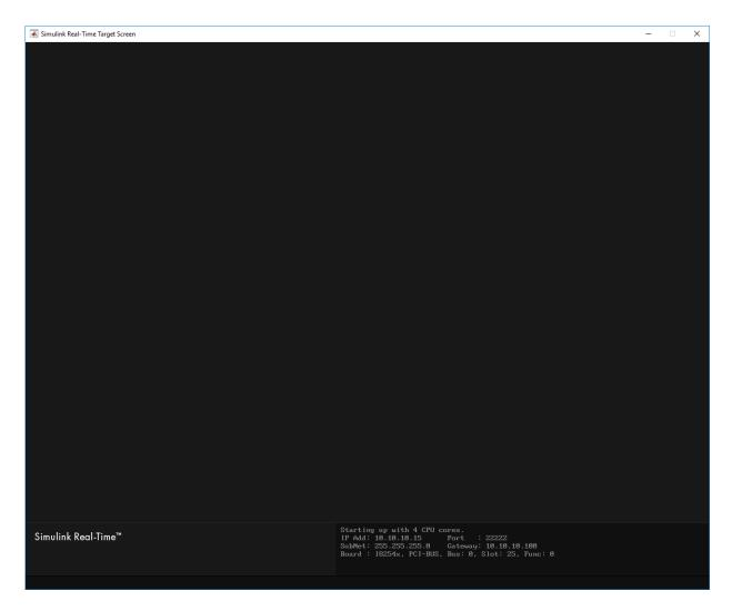
If you have a keyboard attached to the target computer, you can activate that keyboard by typing **C**. Press the **Page Up** and **Page Down** keys to page up and down in the target computer monitor.
