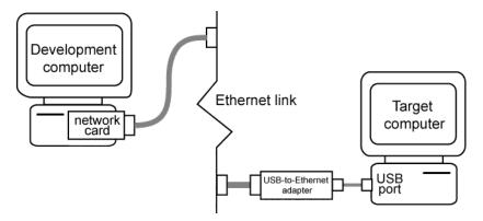
To connect the USB-to-Ethernet protocol interface hardware to the USB port on the target computer:
