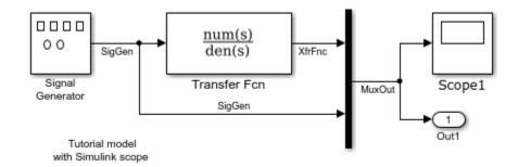
As you go through the tutorial, you transform ex\_slrt\_nrt\_osc into a Simulink Real-Time model configured to build as a real-time application. You then build, download, and execute the real-time application on the target computer.
